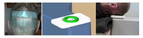
Ergonomic detachable support for underarm measurements (support is fixed to the analyzer)
